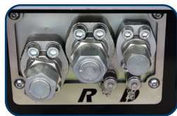
Labeled Hose Ports
