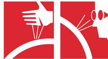
Leaking fluids under pressure can enter the skin and cause serious injury or death. Immediate medical attention is required. Wear goggles. Use cardboard to check for leaks.
