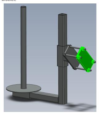
2. Slide the mounting bracket over the main boom of the silt fence installer, approximately 4.5" behind the rear of the side panels.
