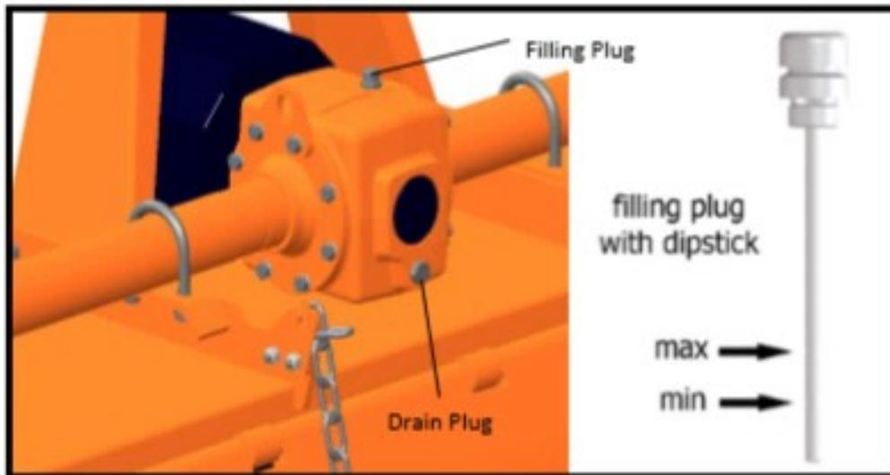
If the sign is below the minimum, fill up oil till restore the correct level.
