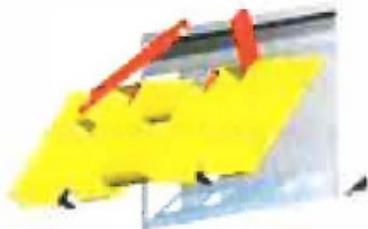
When the top edge of the coupler is seated in the top part of the coupler plate, roll the skid steer tilt function back until the attaching plate is flat against the skid steer coupler. Lock down the coupler levers.
