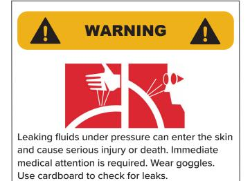
Check condition of all hydraulic components for leaks. Repair as required.
