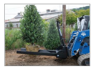
Drive forward and position the tree between the forks and as close to the fork frame as possible. Gently angle the fork inward until the forks contact the tree ball or container. Use the loader arms to raise or lower the tree.
