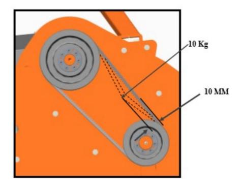
If the deflection is about 10 mm, the tension is correct. If is not so, proceed with the adjustment in the following way (see picture below):
