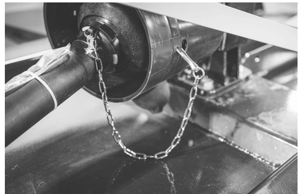
Attach PTO driveline safety chain.
