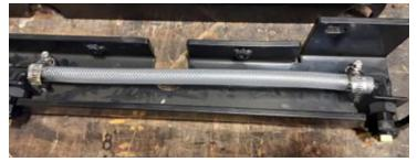
13. Bolt the spray bar halves together.
