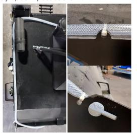
11. Attach the nozzle fittings to the spray bar. Insert the filter, and thread the nut over the spray nozzle.
