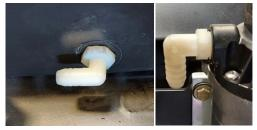
8. Thread the filter and remaining fittings into the pump inlet as shown. Ensure the direction of flow through the filter is towards the pump.
