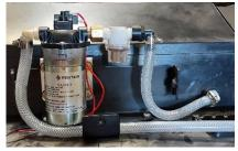
10. Route the hose around the Owner's Manual tube, and loosely zip tie in place as shown.
