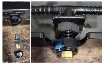
Connect the nozzle fittings with the small hose. Make sure to connect the three–barbed tee in between two of the end nozzles as an inlet (not shown).
