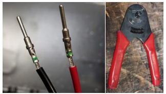
Push pins into Deutsch connector, black on "1" and red on "2" as shown. Pull-test both wires.
