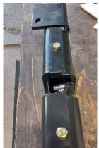
14. Loosely attach the end of the spray bar furthest from the inlet tee. Block up the tee end, and attach the loose end of the hose with a hose clamp. Tighten the hose zip ties. Bolt the spray bar to the hood, and tighten both ends.
